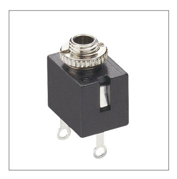
Jack chassis socket acc. to JIS C 6560 JC25P2B, 2.5 mm, 2 poles/mono, with break contact and solder eyes, for back side mounting
