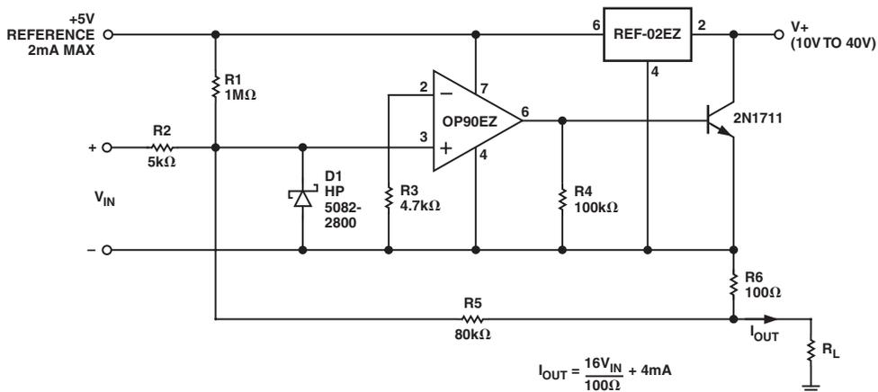
Figure 9. 2-Wire 4 mA to 20mA Transmitter
