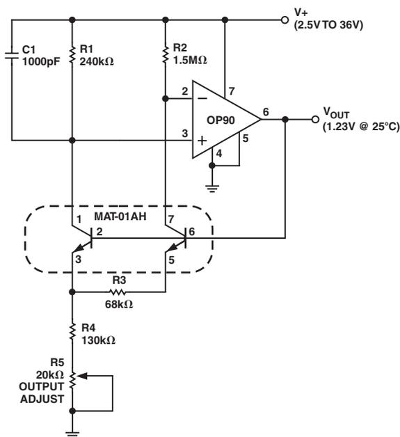
Figure 6. Battery-Powered Voltage Reference
