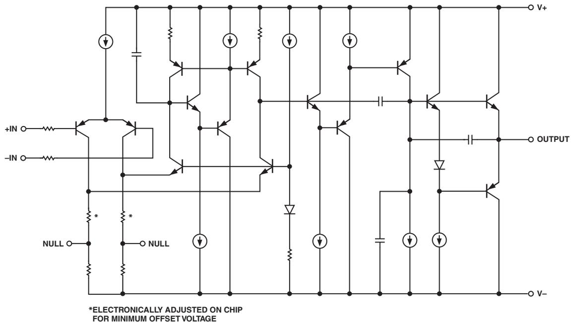
Figure 1. Simplified Schematic
