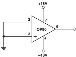
Figure 2. Burn-In Circuit
