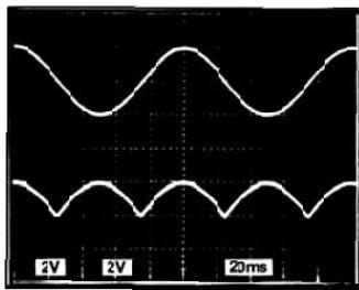
Figure 8. Output of Full-Wave Rectifier with 4 V<sub>p-p</sub>, 10 Hz Input
